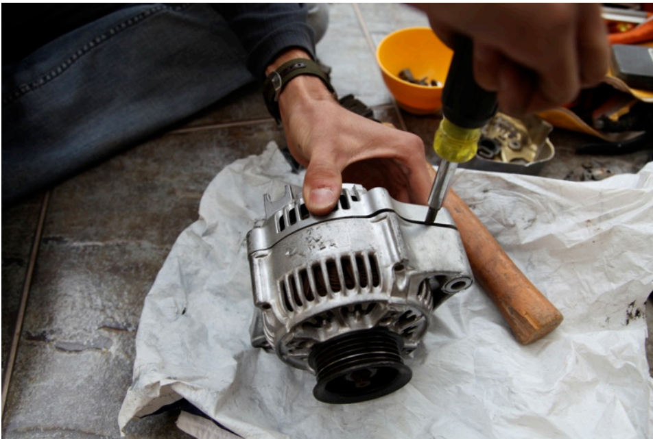
Prying the alternator apart with the five-in-one screwdriver.
