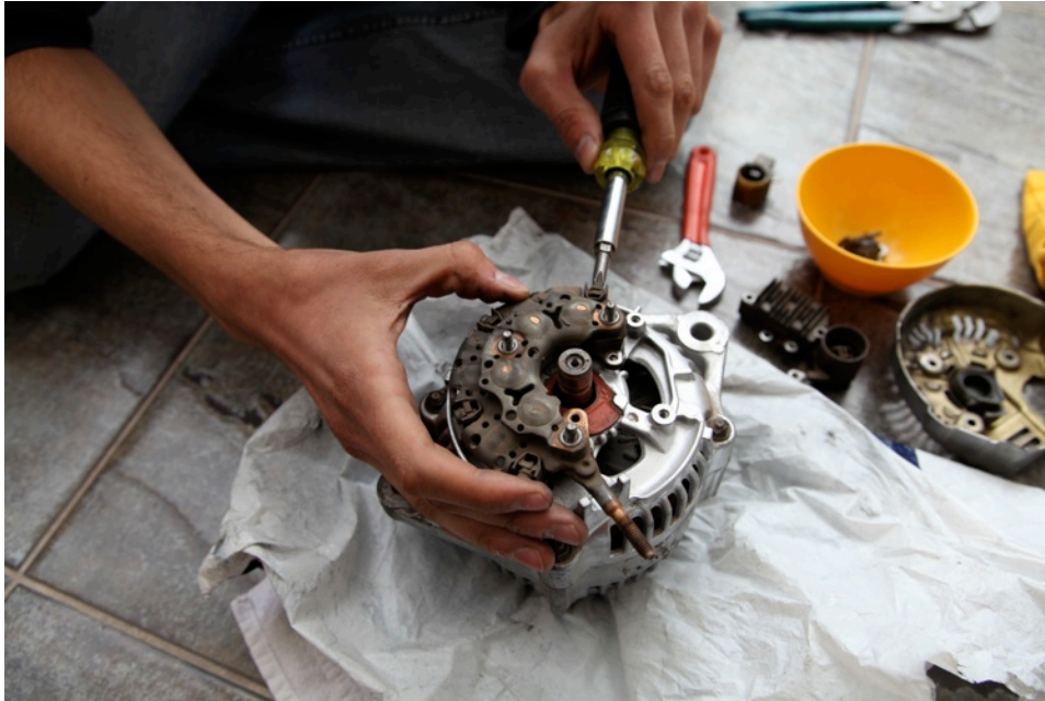
Removing the four screws that connect the rectifier to the stator inside the alternator.
