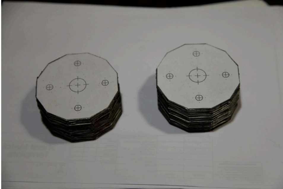
Cores with templates for the four side holes and center hole, ready for drilling.
