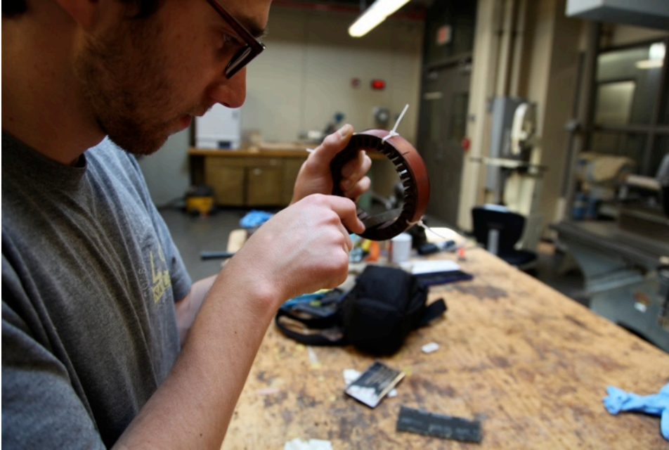
Burs being filed from the stator.
