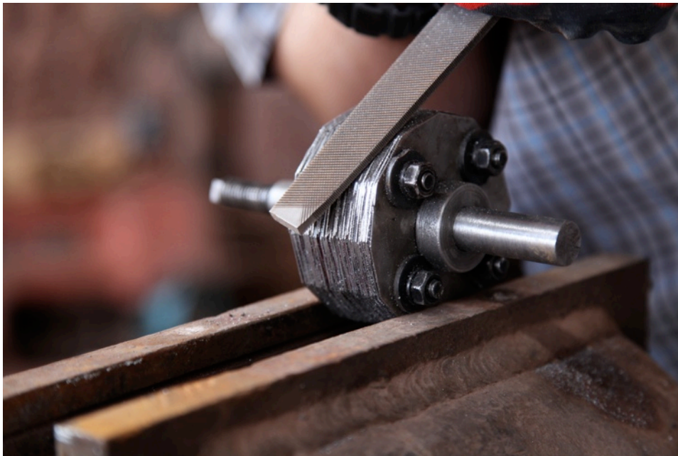
The rotor core being filed to dimension.
