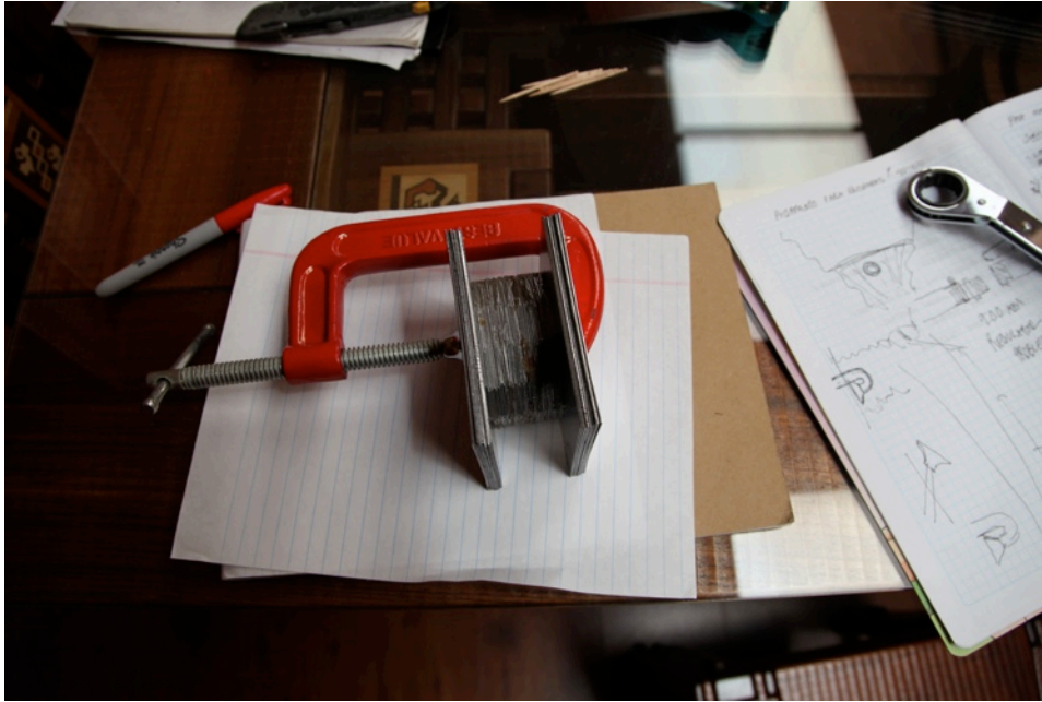
The laminates of the core clamped together.
