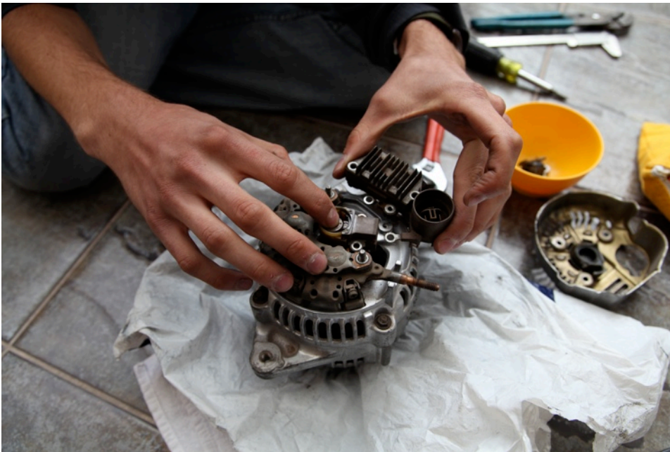
Removing the voltage regulator.
