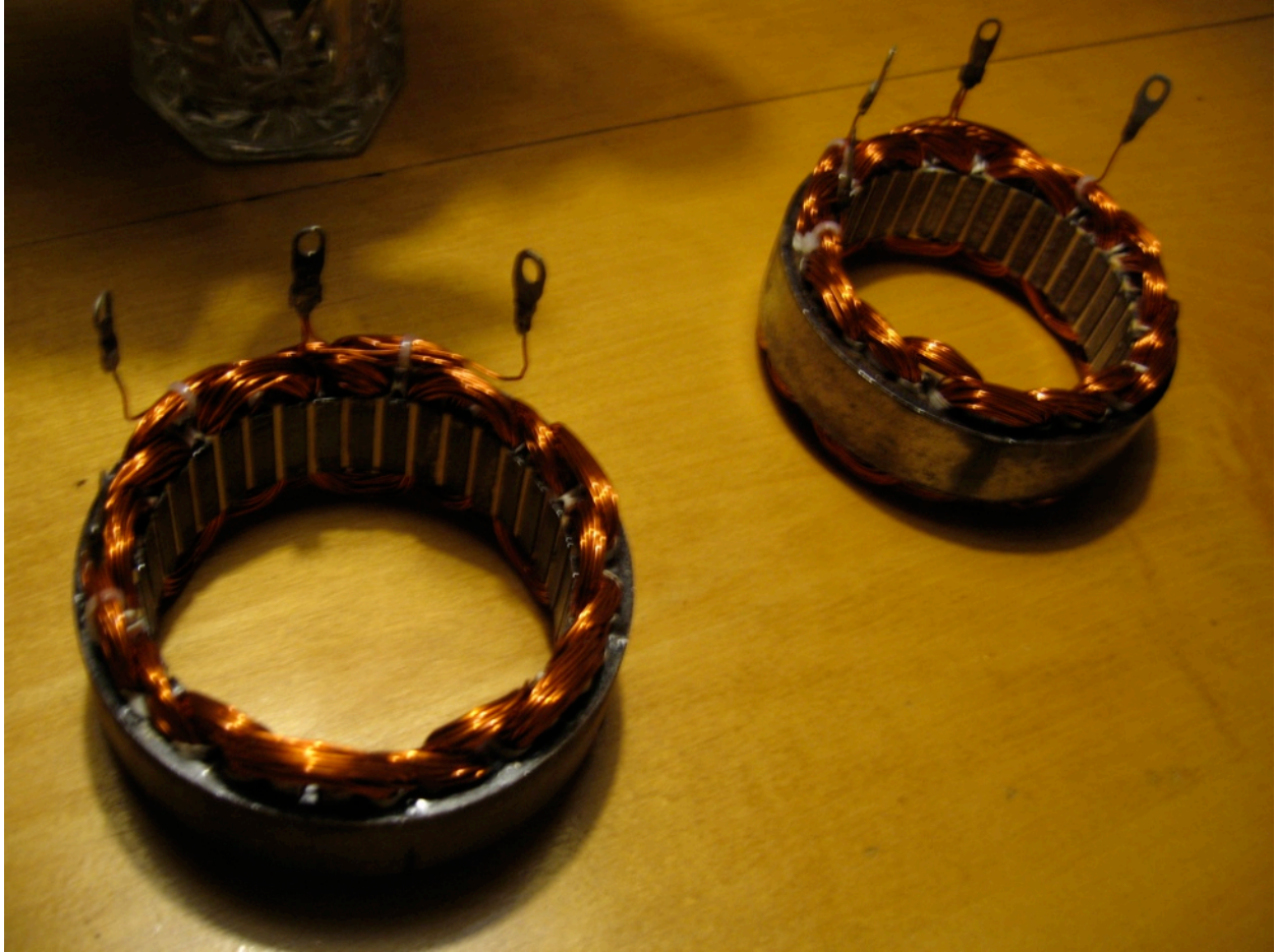
Finished stators with wire lugs reattached to each phase and the common wye connection.
