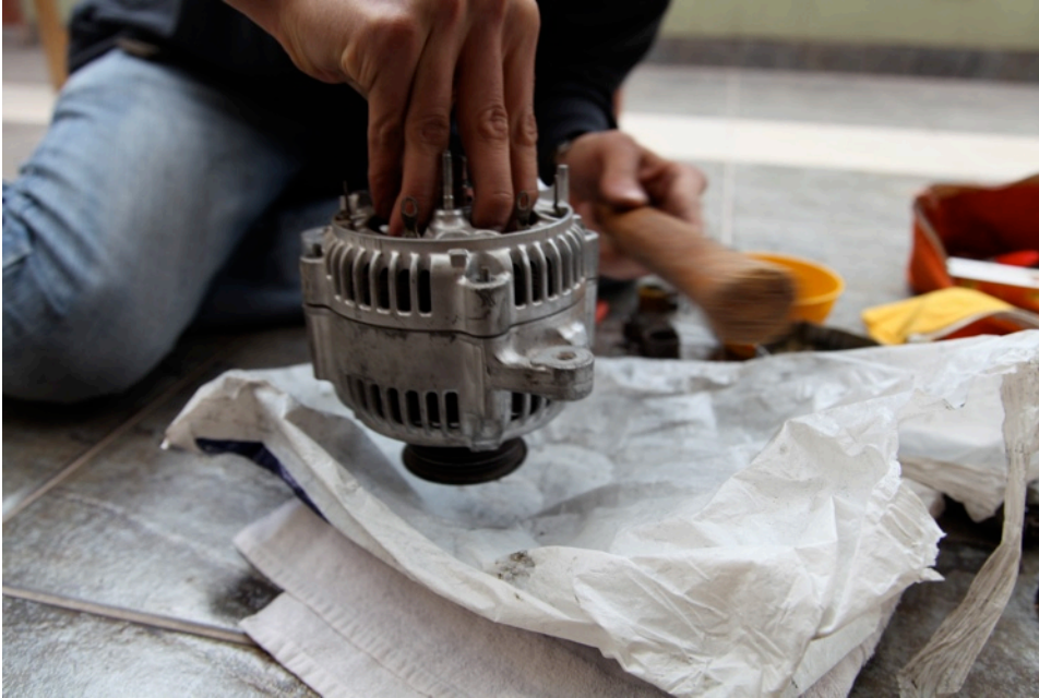
Tapping the sides of the alternator while holding it aloft.
