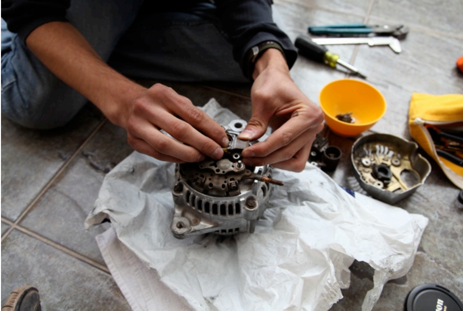
Removing the brush assembly.
