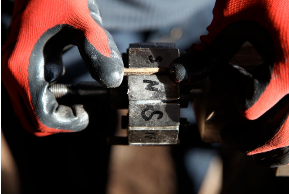
Magnets being applied to the rotor core.
