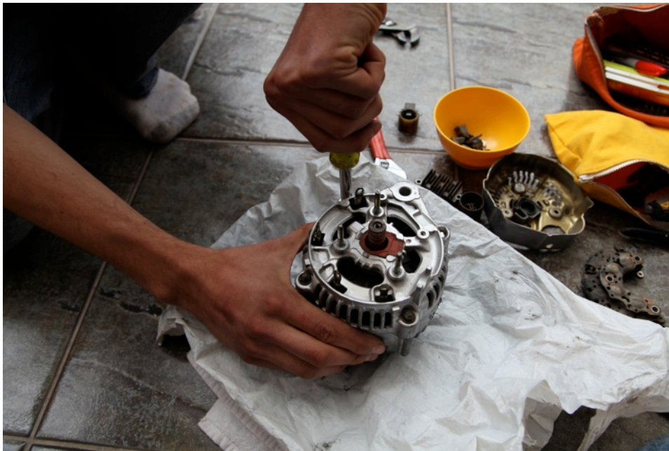
Removing the nuts that hold the front and back of the alternator together.
