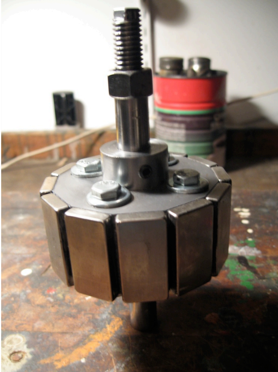
The finished permanent magnet rotor.
