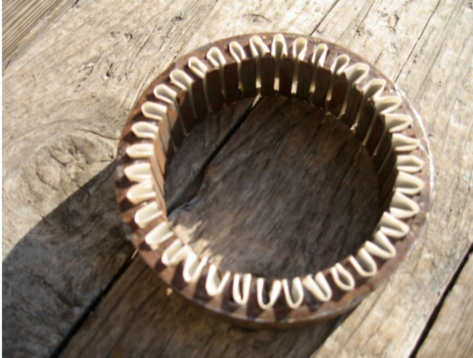
The stator core slots lined with Nomex paper.
