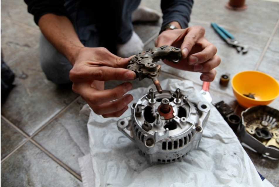
Removing the rectifier from the alternator.
