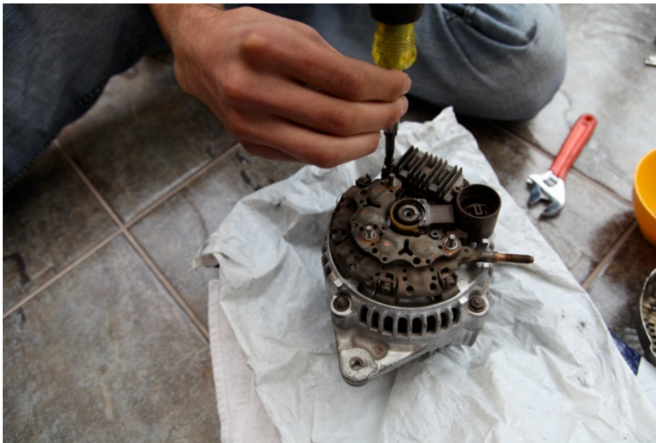
Removing the three retaining screws for the voltage regulator.
