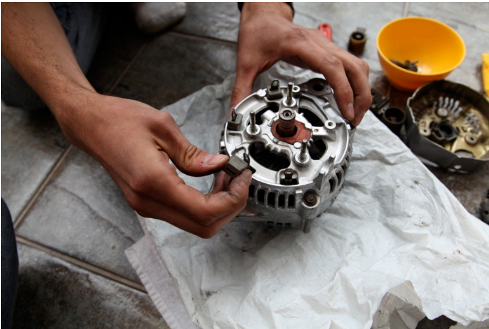
Removing the four rubber insulators from the wires that connect the rectifier to the stator.
