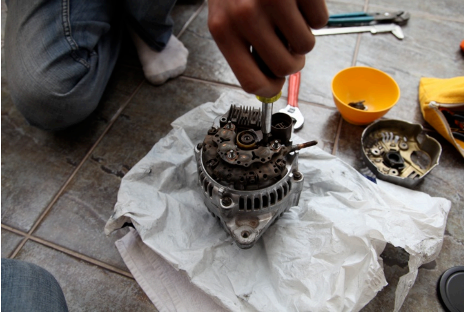
Removing the two screws for the brush assembly.
