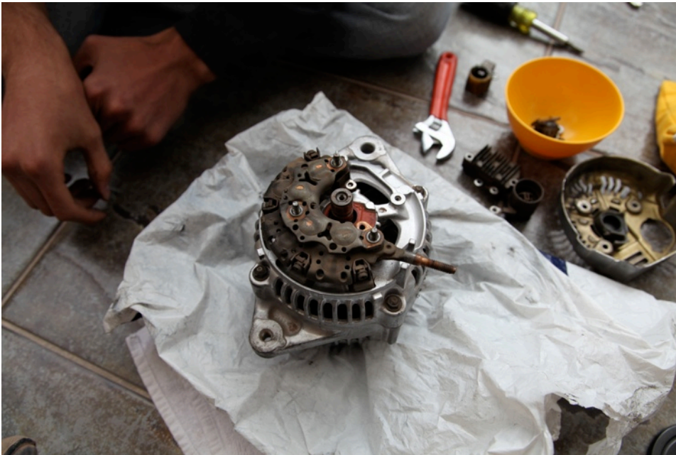
The alternator with the voltage regulator and brush assembly removed.
