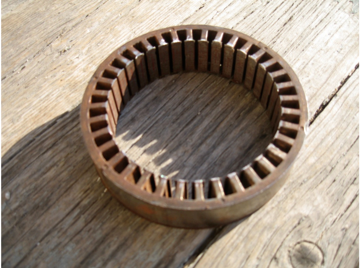
Stator core stripped of factory wire.
